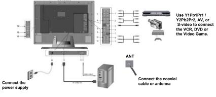
Audio cable connects to PC audio. VGA cable connects to VGA card.
